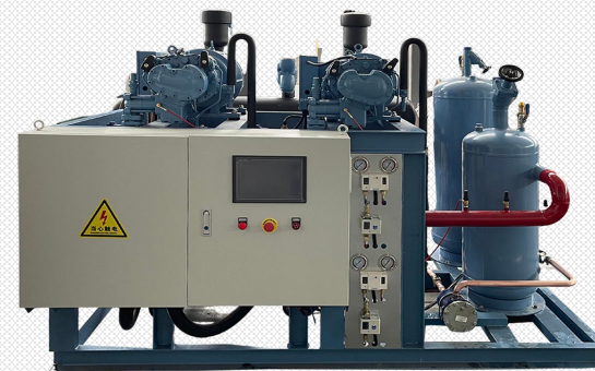
制冷压缩机组 Refrigerating compressor
